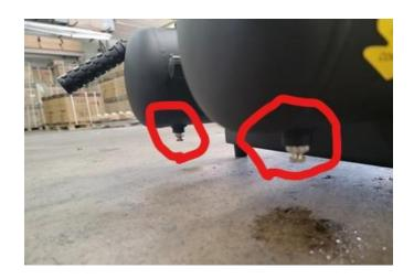
tanks and starts the engine. Once the engine starts make sure to tighten the pressure release valves to build up pressure again.
