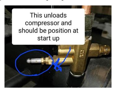
Once the compressor is started flip the switch up or down to load the compressor.
