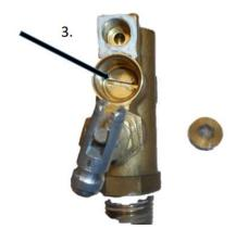
Before installing your new unloader valve, remove the cover for the bypass valve and add a drop or two of oil on the screw edge. Do not attempt to remove the screw. See that the oil flows around the screw head. Ensure there is no dirt or debris in the area. Then exercise the valve a few times by pressing on it with a flat tip screwdriver. You should feel it move in and out freely. Reinstall cover and tighten.
